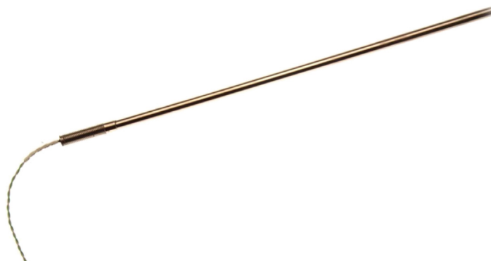
Figure 14.8 Typical probe encasing a thermocouple.
